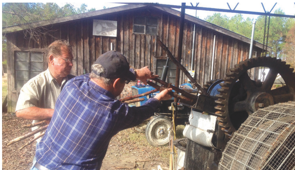
Staff photo Marvin and Wilbur Russ, owners of Old Plantation Syrup in Florence County, feed raw sugarcane stalks into a grinder that extracts the juice, which flows into the shed behind them.
