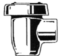
Atmospheric Vacuum Breaker
